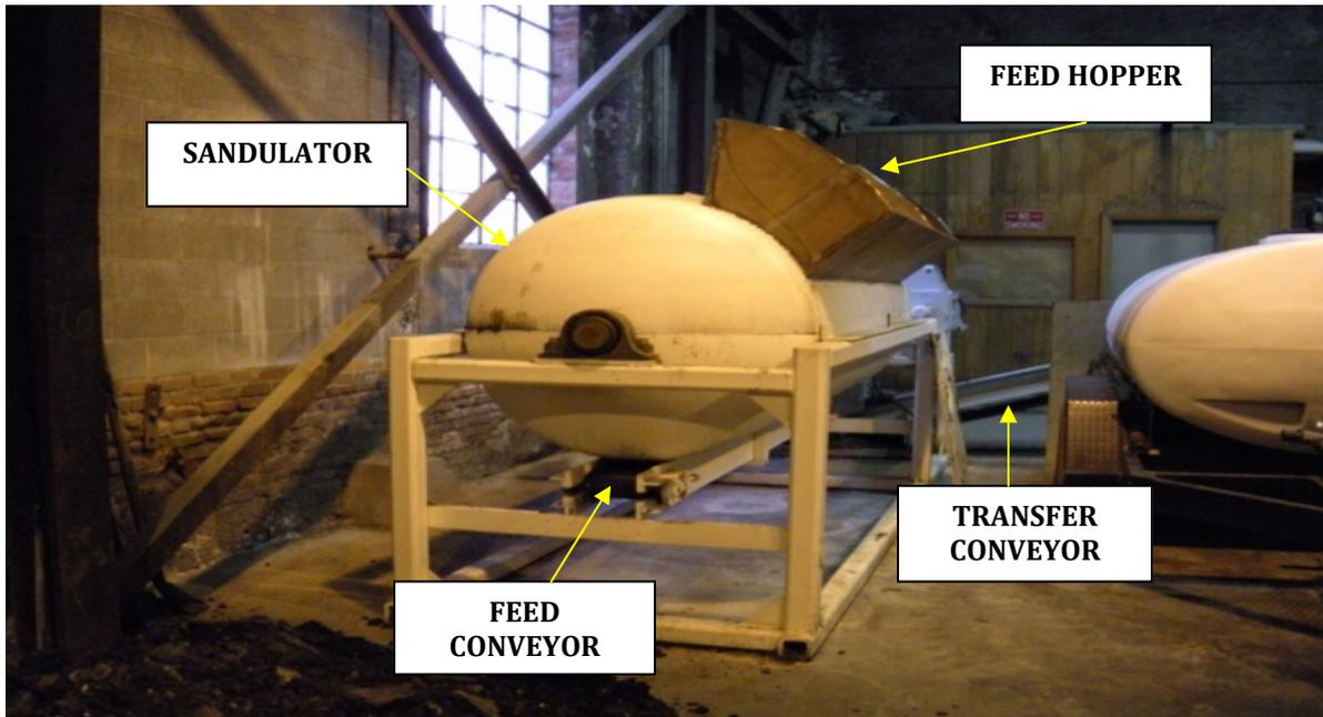
**(2 & 3) Sandulator** – This device is used to break up any lumps of raw oil sands so as to make it “flowable” and the associated load cells permit the feed rate to the slurry tank to be measured.
