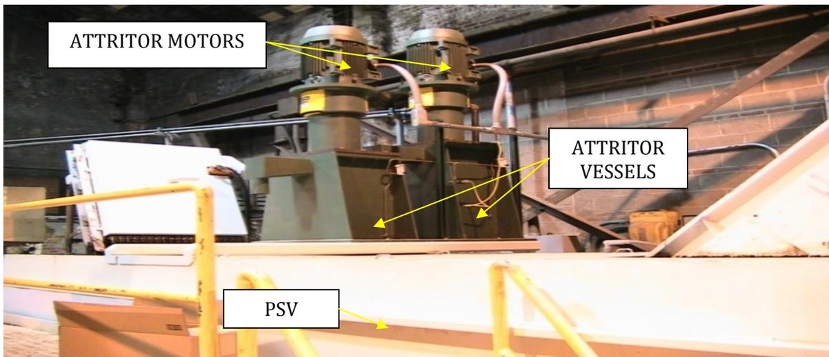
**(5) Attritors** – These high speed/high shear mechanical devices separate the bitumen from the solids and fines. The chemistry in the PSV prevents the re-association of bitumen, solids, and chemistry.
