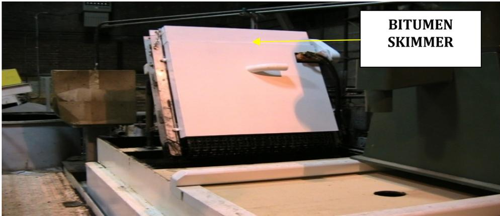
**(7) PSV Bitumen Tank** – Floating bitumen is collected in the PSV by means of a skimmer and discharged into a heated holding tank before being pumped to the polishing unit, if required.
