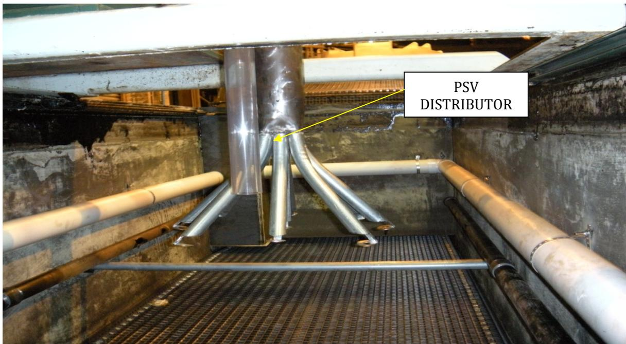
**(6) Primary Separation Vessel** – This vessel continuously receives the product from the attritors. After a short settling time, the mixture stratifies into three distinct layers: 1) the bitumen floats to the top; 2) middlings, primarily made up of CAC-24 with some suspended fines, settles in the middle and; 3) all of the solids, with most of the fines drop to the bottom.
