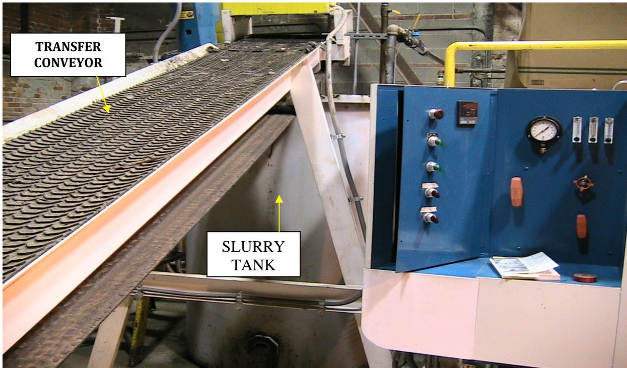
**(4) Slurry Tank** - This is the first place where raw oil sands are mixed with the chemistry, CAC-24. This is a mechanical mixing device that forms a slurry, which is pumped to the **attritors**. The mixture of CAC-24 to oil sands is 70/30 to 50/50.
